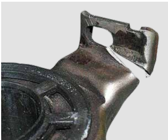
RELEASE FORK MOUNT ON THE RELEASE BEARING IS BROKEN
