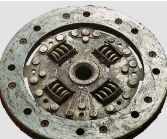
CLUTCH LININGS ARE COVERED IN EXCESS GREASE
