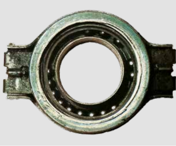
CONTACT BUSHING AND BALL BEARING ON THE RELEASE BEARING ARE DESTROYED
