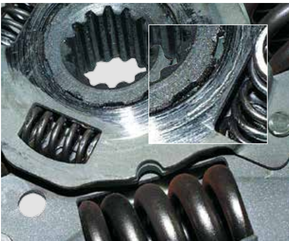
CONTACT TRACKS ON THE FIRST STAGE DAMPER
