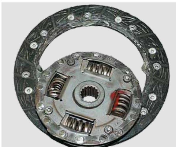
DISC ASSEMBLY IS BROKEN
