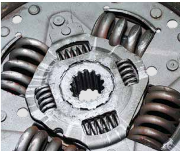
HUB PROFILE HAS BEEN INCORRECTLY GREASED
