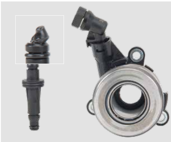
CSC BURSTS DIRECTLY AFTER INSTALLATION
