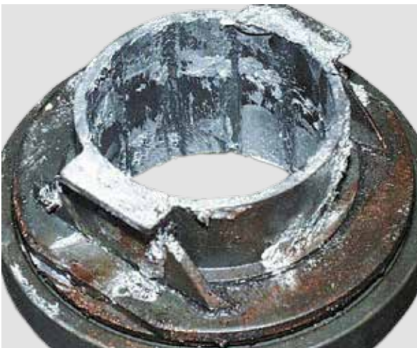
RELEASE BEARING HAS BEEN INCORRECTLY GREASED
