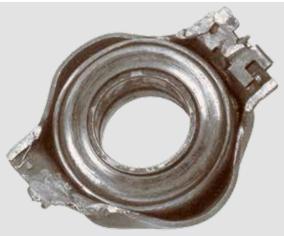
HOUSING OF THE RELEASE BEARING IS DEFORMED
