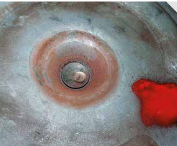
OFF-CENTER CONTACT TRACK IN THE RELEASE SPRING (VW CLUTCH SYSTEM)
