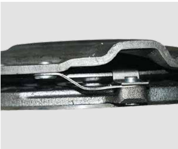
TANGENTIAL LEAF SPRING IS BENT
