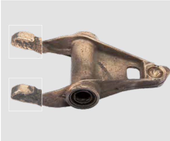
RELEASE FORK TIPS ARE WORN (PULL-TYPE CLUTCH)
