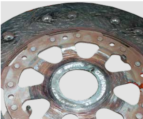
HUB OF THE CLUTCH DISK IS BROKEN
