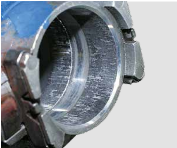
TRACKS IN THE RELEASE BEARING SLEEVE
