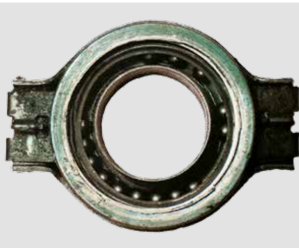
CONTACT BUSHING AND BALL BEARING ARE DESTROYED
