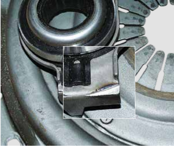
CONTACT TRACKS ON THE CLUTCH COVER AND RELEASE BEARING
