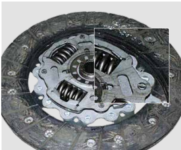
FRICITION LINING ON THE INNER RING IS OILY/ GREASY
