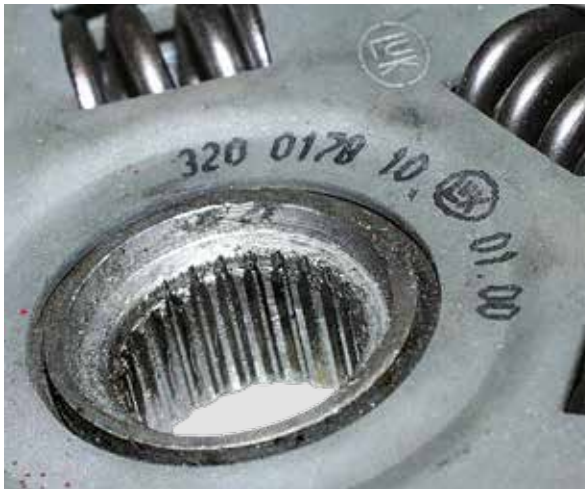
HUB PROFILE IS DAMAGED
