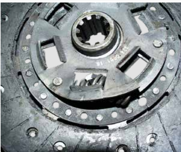
TORSIONAL DAMPER IS BROKEN
