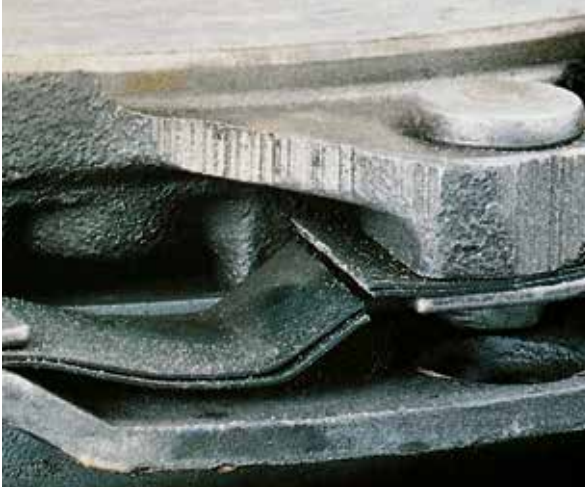
TANGENTIAL LEAF SPRING IS BROKEN
