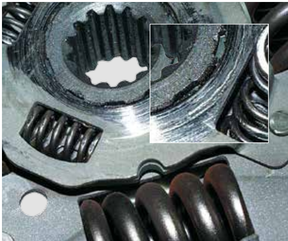
CONTACT TRACKS ON THE FIRST STAGE DAMPER OF THE CLUTCH DISK
