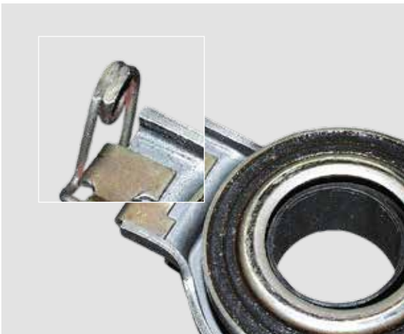
CONTACT TRACKS ON THE FORMED SPRING
