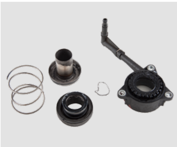
MECHANICAL DAMAGE TO THE CSC
