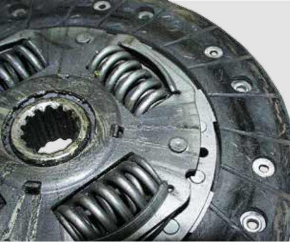
CLUTCH LINING IS OILY
