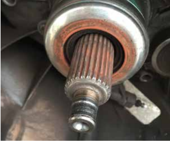
PILOT BEARING IS DEFECTIVE
