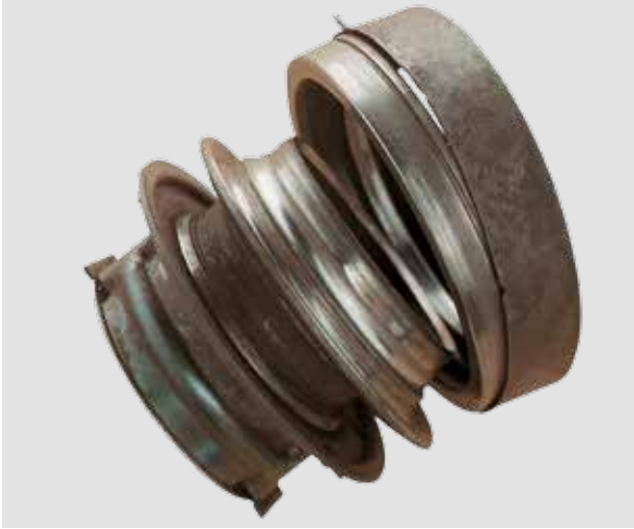
FLANGE ON THE RELEASE BEARING IS WORN THROUGH
