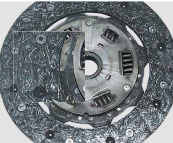
CLUTCH LINING IS WORN DOWN TO THE RIVETS
