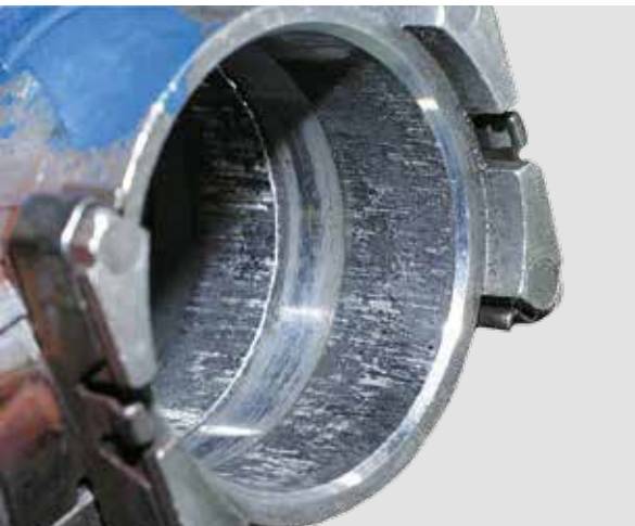
RELEASE BEARING IS STIFF, SIGNS OF WEAR ARE VISIBLE
