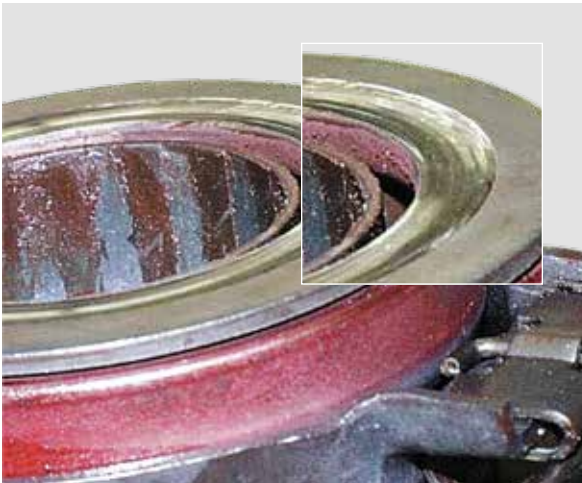
SIGNS OF WEAR VISIBLE ON THE THRUST RING OF THE RELEASE BEARING
