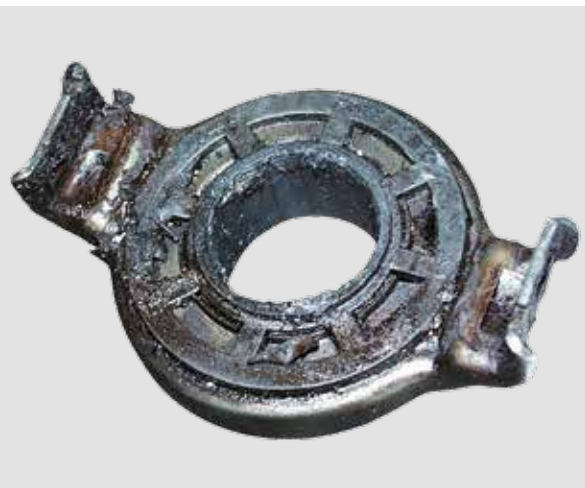
RELEASE BEARING SEATING IS WORN
