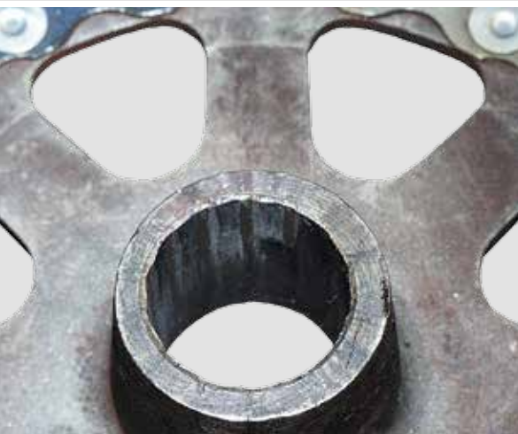
HUB PROFILE IS COMPLETELY MISSING
