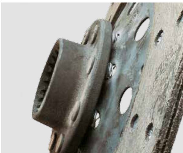
CLUTCH DISK HAS BECOME SAUCER-SHAPED
