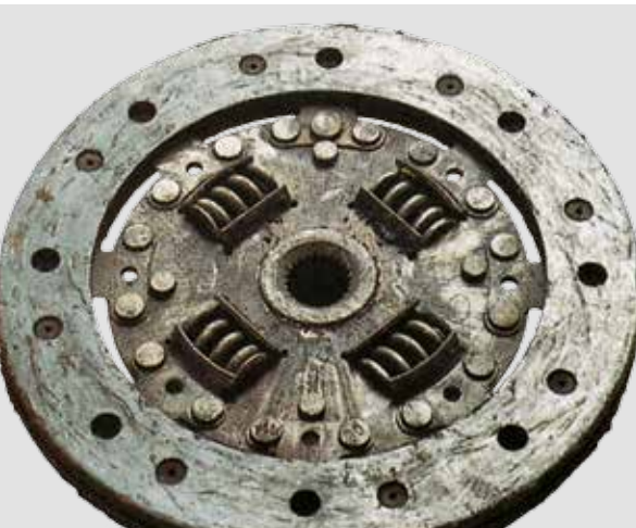
CLUTCH LINING IS OILY
