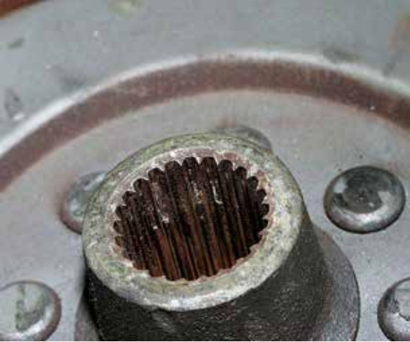
HUB PROFILE IS DEFORMED, TAPERED GEARING PROFILE TORSIONAL DAMPER IS DESTROYED
