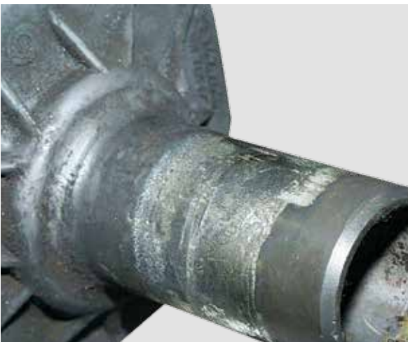
SIGNS OF WEAR VISIBLE ON THE GUIDING SLEEVE
