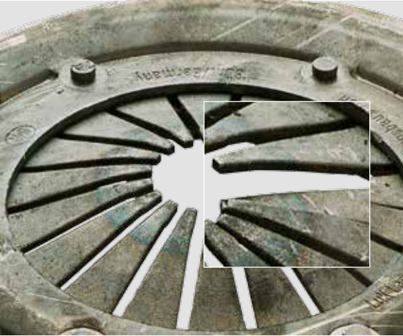
DISK SPRING TIPS ARE BENT
