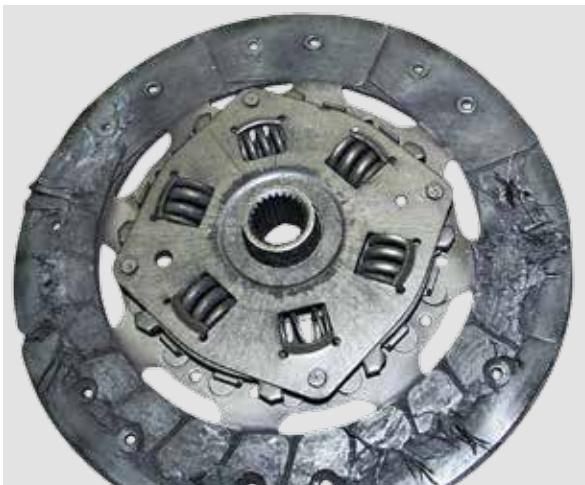
LINING IS BURNT OR HAS WORKED LOOSE
