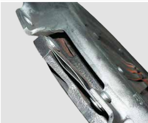
TANGENTIAL LEAF SPRING IS BENT
